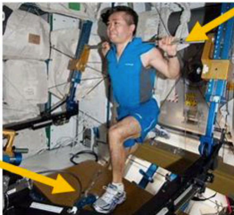
Figure 3. ISS ARED – Squat Overview of ARED capabilities
